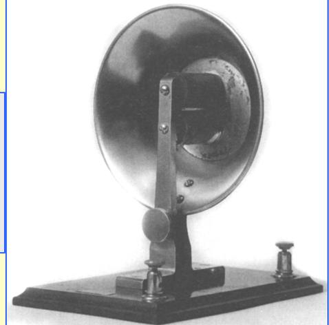
receiver," although it clearly was conceived to operate by magnetostriction. This ambiguity is reflected in [14], in which the author, after noting that this instrument was equipped with a "*diaphragm*, originally an ordinary shoe-blacking box, supported near the poles of the electromagnet" (*italics added*), concludes that this receiver "anticipated the design of the modern telephone receiver." One finds similar statements in [13].
