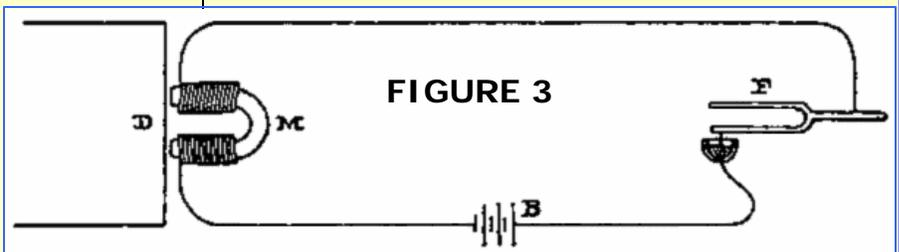
**Cross's Electromagnetic Receiver (1872) Derived from Pickering's (1869) Tin-Box Receiver**
